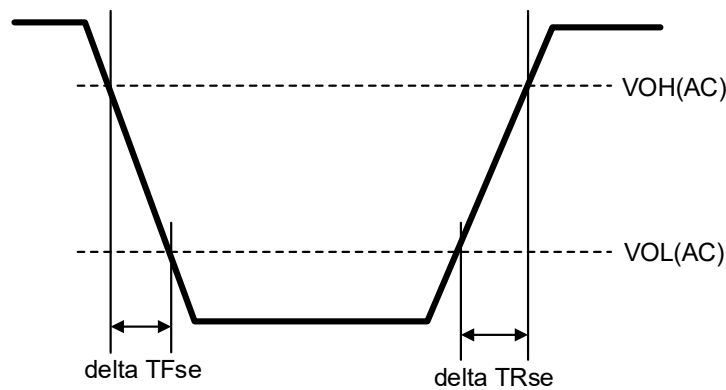
Figure 8-2. Single-ended Output Slew Rate Definition
